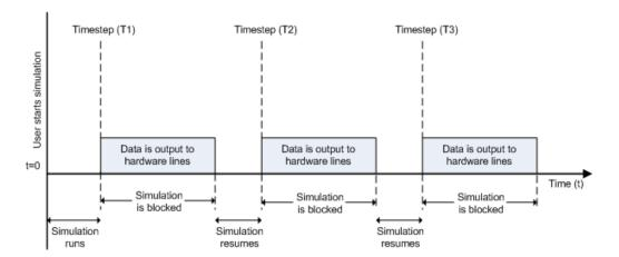
At the first time step (T1), data is output to the selected hardware lines. The simulation does not continue until data is output to all lines.
