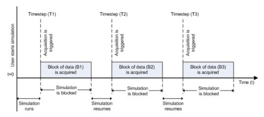
At the first time step (T1), the acquisition is initiated for the required block of data (B1). The simulation does not continue until B1 is completely acquired.
