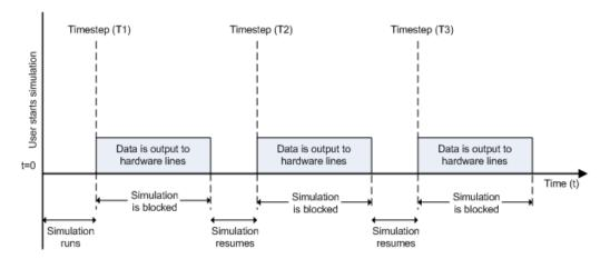
At the first time step (T1), data is output to the selected hardware channels. The simulation does not continue until data is output to all channels.
