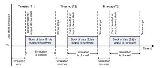
At the first time step (T1), data output is initiated and the corresponding block of data (B1) is output to the hardware. The simulation does not continue until B1 is output completely.
