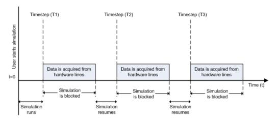
At the first time step (T1), data is acquired from the selected hardware channels. The simulation does not continue until data is read from all channels.
