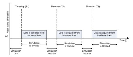
At the first time step (T1), data is acquired from the selected hardware lines. The simulation does not continue until data is read from all lines.
