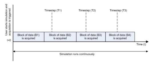
Scenario 2 shows the case when data acquisition speed outpaces simulation speed. At the first time step (T1), the required block of data (B1) has been completely acquired. Therefore, the simulation runs continuously.
